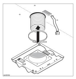
Secure the ducting to the mounting plate using a hose clip.
